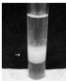
Fig. 1. Emulsions produced by B. subtilis M14 supernatant when added to hexadecane
