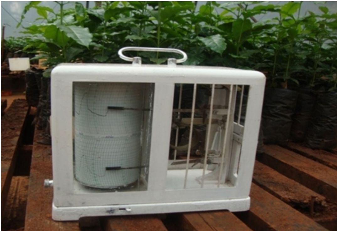
Plate 1. Thermo-hygrograph used to record temperatures and RH
