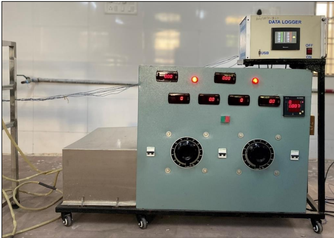
Fig. 5. Control panel for continuous ohmic heater
