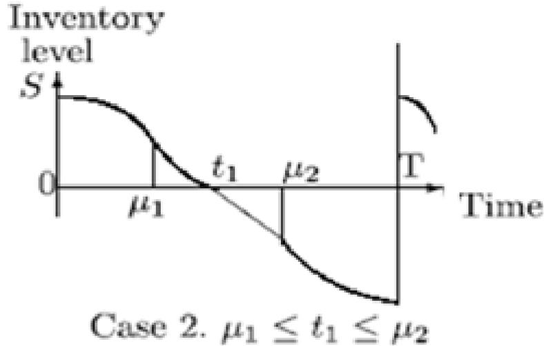
Figure 2. Graphical representation of inventory level over the cycle for case 2.
