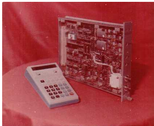
Fig. 8. The “golden” self-correcting 18-digit ADC
