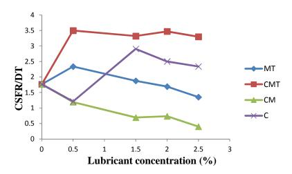
Fig. 5. Representative plot of CSFR/DT versus lubricant concentration
