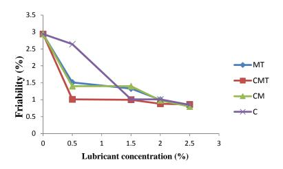
Fig. 3. Representative plot of % friability versus lubricant concentration
