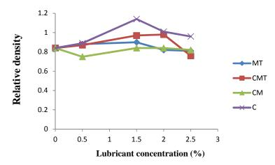
Fig. 1. Representative plot relative density versus lubricant concentration
