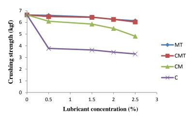
Fig. 2. Representative plot of crushing strength (kgf) versus lubricant concentration
