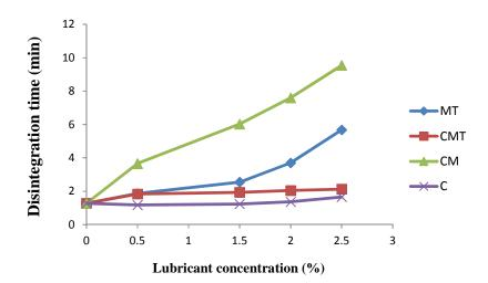
Fig. 4. Representative plot of disintegration time versus lubricant concentration
