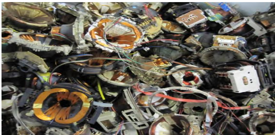
Fig. 1. Focusing and deflecting coils of dismantled CRTs (Source: Manhart et al. 2011 [9])
