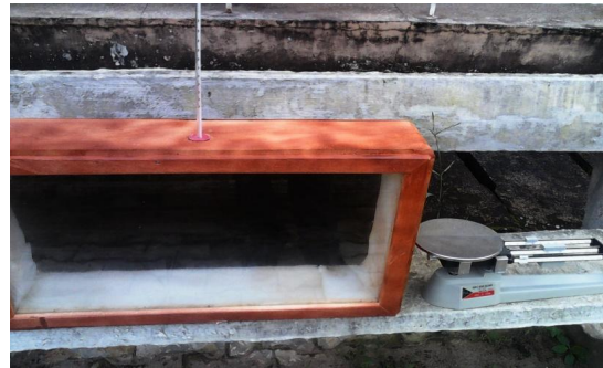
Fig. 1. Prototype solar dryer box
