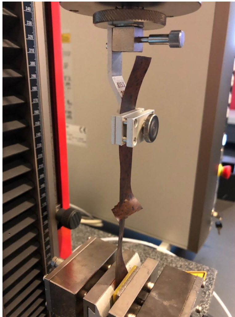
Fig. 2. Image of the set-up for tensile testing (one of the “glass samples”)
