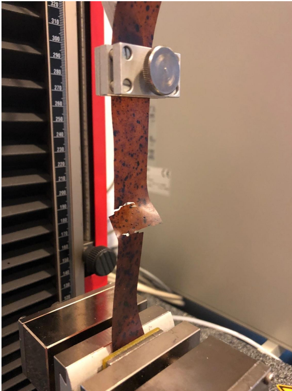
Fig. 4. Image of a tensile sample during breakage (one of the “glass samples”)
