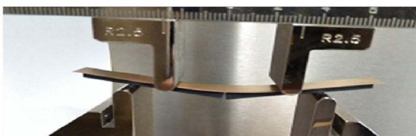
Fig. 9. Mold/copper beam with symmetrical propagation of interface delamination using the new setup after anvil alignment and increase in anvil distance
