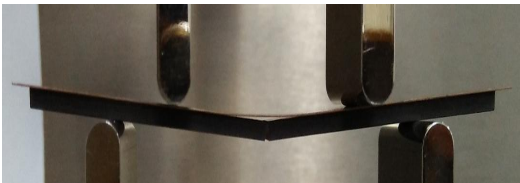
Fig. 9. Mold/copper beam with symmetrical propagation of interface delamination using the new setup after anvil alignment and increase in anvil distance
