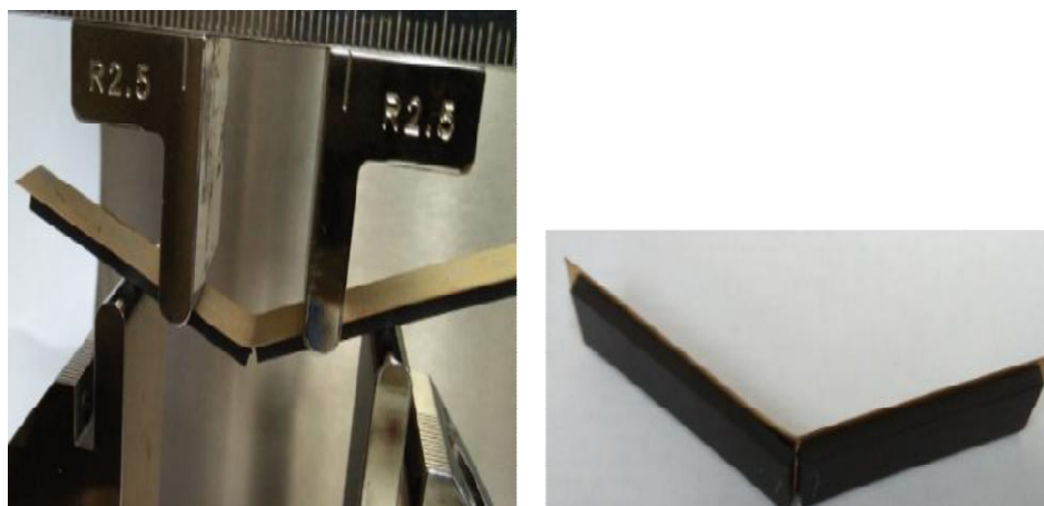
Fig. 6. Mold/copper beam deformed plastically
