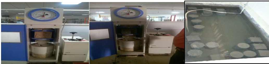
Fig. 5. Compressive strength test machine CTM and curing of cubes, cylinder, beams
