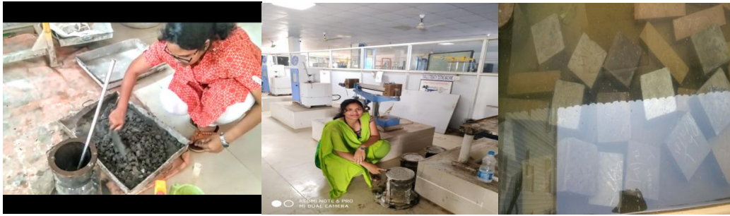
Fig. 4. Mixing casting and testing of curing of SCBA + Siali Ash cubes concrete
