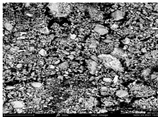
Fig. 4. SEM images of acid-activated Achalla clay (ACAC) (@100 μm)
