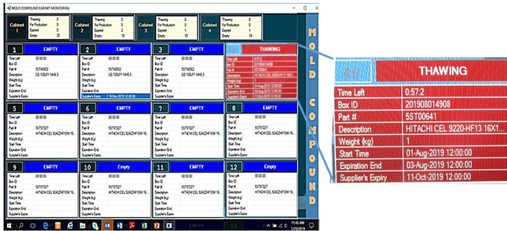
Fig. 15. Mold compound cabinet monitoring system
