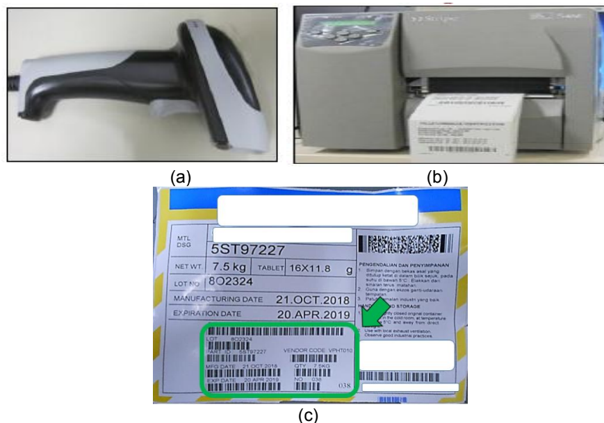
Fig. 10. a) Barcode scanner, b) Barcode printer and label sticker, c) Mold compound supplier label
