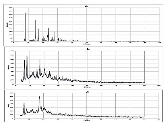
Fig. 3. X-ray diffraction of gabapentin free drug (a), gabapentin with HPMC (b), gabapentin with HPC(c)
