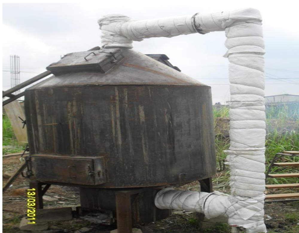
Fig. 1. The first homebuilt biochar reactor
