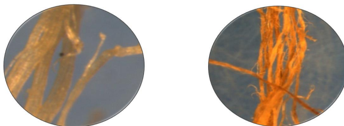
Fig. 3. Microscopic structure of ashoka fibres
